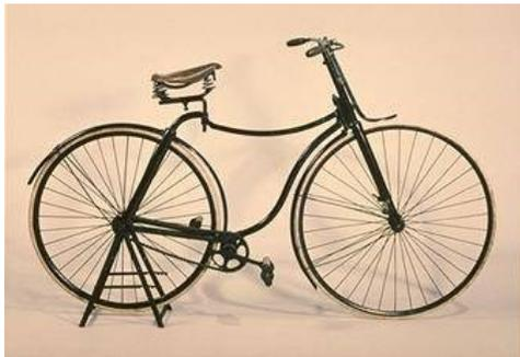
The bicycle featured two wheels of the same size and a chain drive to the rear wheel.
